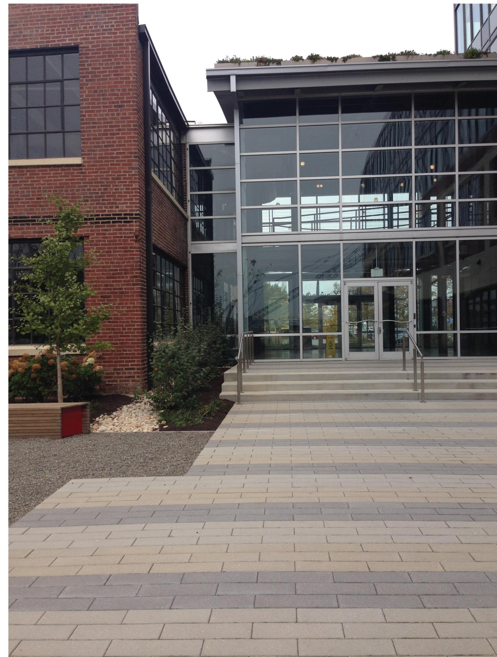
BANDED CONCRETE UNIT PAVERS
