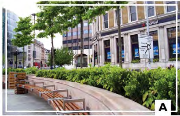
Retaining walls providing seating
